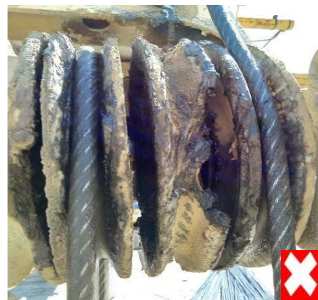
Figure (4): A Structural Issue (Needs Mechanical Intervention)
