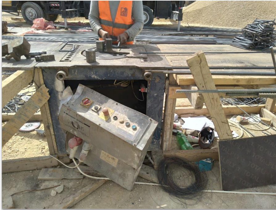
Figure 12: Unsafe Control Panel for Rebar Bending Machine
