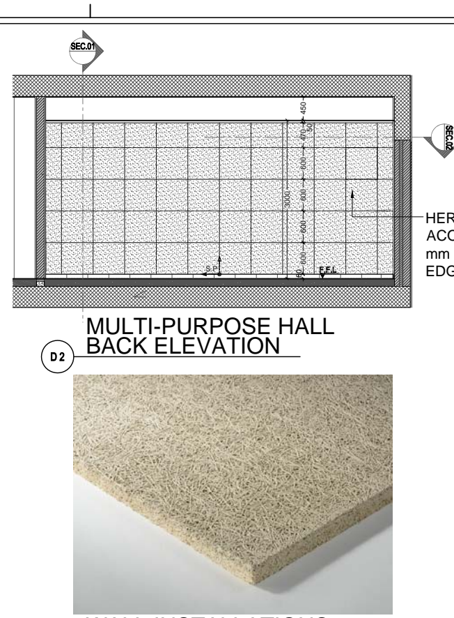
D3 WALL INSTALLATIONS WOOD WOOL ACOUSTIC PANEL COLOR IS SUBJECT TO ENGINEER APPROVAL.
